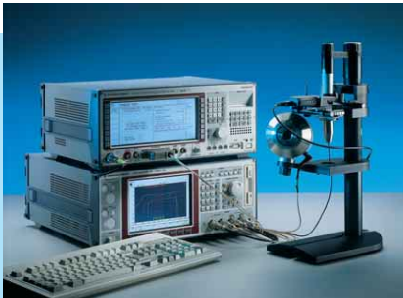
A member of the CMD family used in an audio application with the Rohde&Schwarz Audio Analyzer UPL and artificial ear
